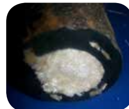
Load bearing fibres protected by thick, black rubber skin
