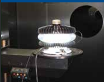
Precision light measurement with Sealite's goniophotometer
