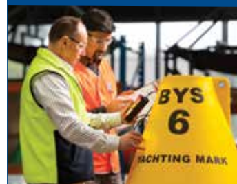
The wall-thickness of each buoy is measured in critical areas by ultrasound
