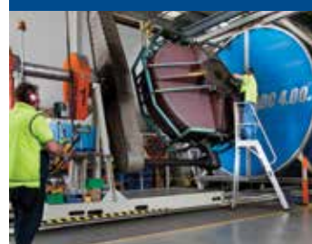
Sealite's marine buoys are manufactured using state-of-the-art rotational moulding equipment
