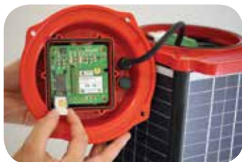
GSM module, SIM card & electronic hardware
