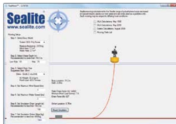
Mooring solutions are calculated using Sealite's advanced mooring calculator
